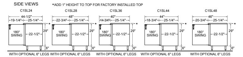
Note: Available with compressor left or right. Compressor left model shown.
