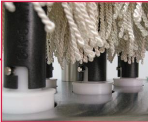
Removable polishing heads are machine washable and easily re-installed.
