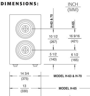
MINIMUM CLEARANCE REQUIRED FROM UNIT TO THE NEAREST COMBUSTIBLE OBJECT. **BACK** SIDE BOTTOM TOP NA 1 4 1 (25) (25) (102)NA
